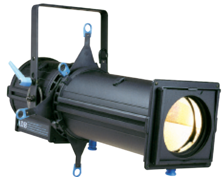
DSN 105 11° - 23° - 1000/1200 W Zoom Profile with Condenser Optics
