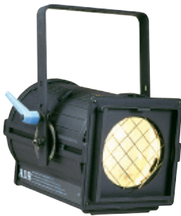
C101 10° - 65° - 1000/1200 W Ø 150 mm Plano-convex Lens
